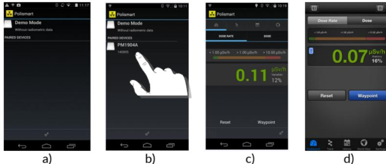
*Figure 2. Connecting PM1904A to mobile devices*
