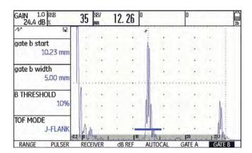
To change the setting of a function, you have to select the function first and then press one of the selector keys next to the display screen.
