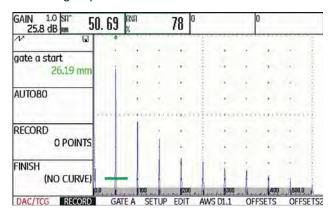
Select the function gate a start and position the gate A on the first DAC echo.
