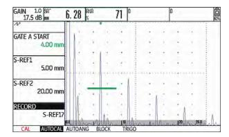
Position the gate on the second calibration echo and record the second calibration echo.
