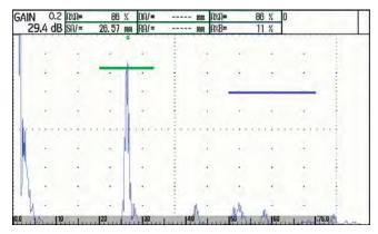
The gain and the adjusted dB step value are always shown in the top left corner of the display screen. The access to all other instrument functions is disabled in the zoom mode of the A-scan display.
