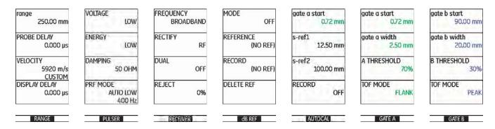
To change between the first and the second operating level press **Home** key for 2 seconds.
