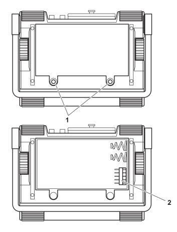
Place the battery in the battery compartment so that the marking faces upwards and the contacts are pushed against the connector pins (2).
