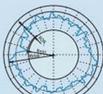
$$RON_N = R_{max} - R_{min}$$
