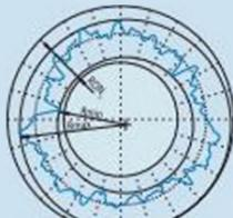
$$RON_M = R_{max} - R_{min}$$
